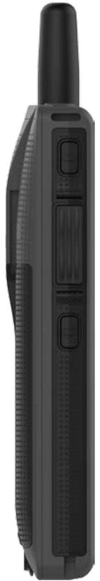
Tactilon Dabat may look like a regular fully rugged smartphone, but it is ground-breaking: it also offers the special multi-purpose push-to-talk buttons familiar from Airbus TETRA radios. It is therefore comfortable in even prolonged use.
